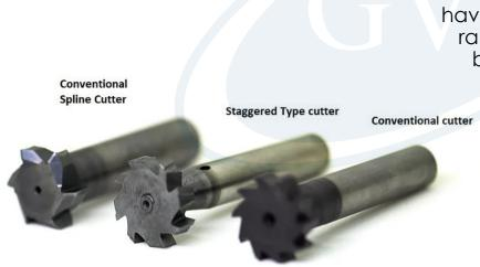
Staggered cutters tend to have excess positive radial rake (leading to a poor backed cutting edge) in the end or low positive radial rake (leading to poor cutting action) in the start based on the alternating helix angle. This can be avoided by slow increase in the starting point, peak in the middle and back to nominal value in the end point, i.e. at point of low axial rake there is high radial rake to compensate the cutting action and vice versa.
